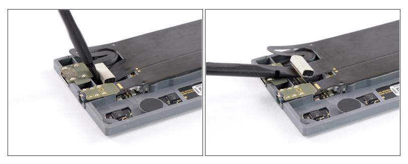
• Use the spudger to disconnect the flex cable from the encoder board.
