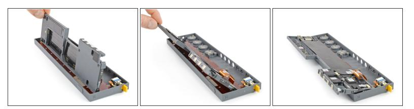
• Flip the midframe over to gain access to the flex cable connector underneath.
