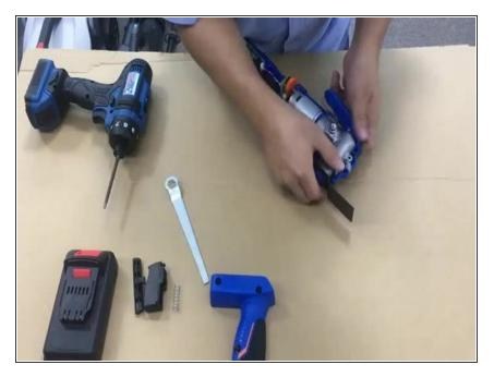
• Remove the motor head.
