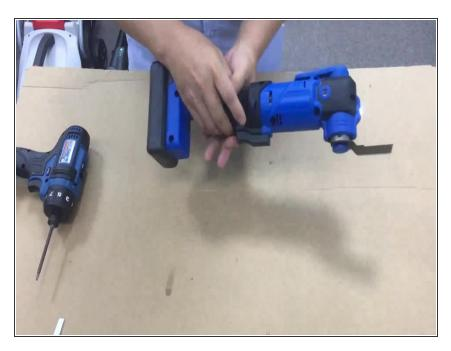
• Remove the battery. Remove the screws on the tool body.
