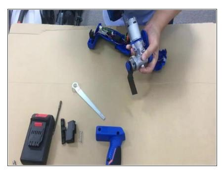
• Disconnect the motor from the grinding head.
