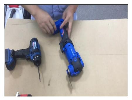
• Disassemble the tool body. Remove the grinding head.
