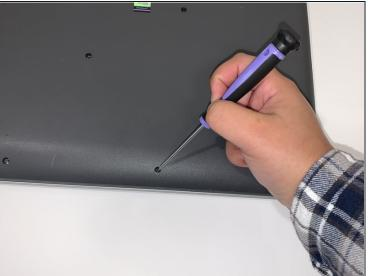
• Remove fourteen 7mm Phillips #00 screws from the back panel.
