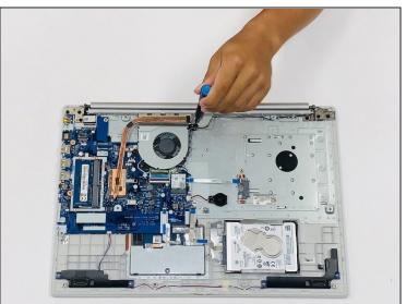
• Remove five 7mm Phillips #00 screws from the cooling fan.
