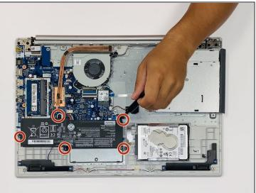
• Remove five 7mm Phillips #0 screws from the battery holder.
