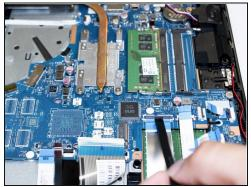
Unplug the eight ribbon cables by flipping up the "easy-on" connector using the flat end
