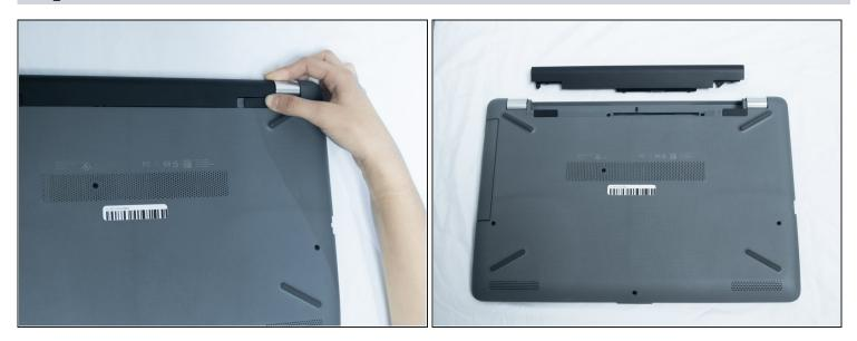
• Slide the Battery release slider towards the battery while pulling the battery out.
