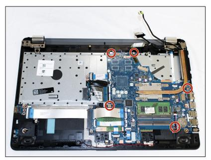
• Use a Phillips #0 screwdriver to unscrew the five 3.3mm screws from the motherboard.
