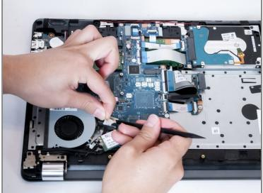
• Carefully unplug the LCD connector using a plastic spudger.
