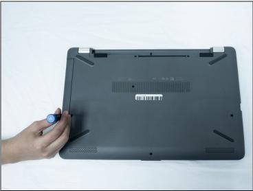
• Use a Phillips #1 screwdriver to remove the six 10.5 mm screws visible on the bottom of the laptop.
