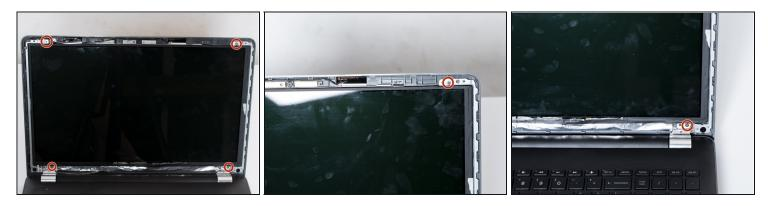
• Use a Phillips #0 screwdriver to unscrew the four screws at the top corners and the two screws at the bottom corners.
