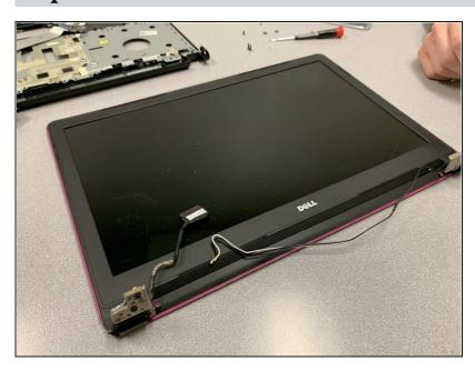
Remove the screen from the lower assembly by lifting it up from the now disconnected right and left hinges.
