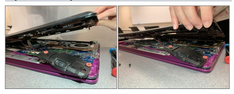
• The speakers may be removed from the computer base by unattaching from the computer base or disconnecting the cable and leaving the speakers on the computer base.
