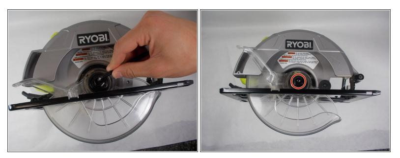
Use the  $7^{"}/32$  allen key to loosen the  $5/16-18 \times 9/16$  in. blade screw.
