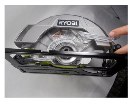
• Remove the blade from the saw.
