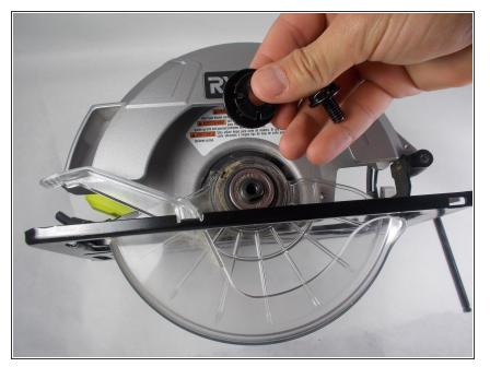
Remove the 5/16-18 x 9/16 in. blade screw, spring washer, and the outer blade washer.
