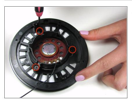
With a #0 phillips head, unscrew the three, 1 cm screws which are holding the driver (red wafer) in its bracket.
