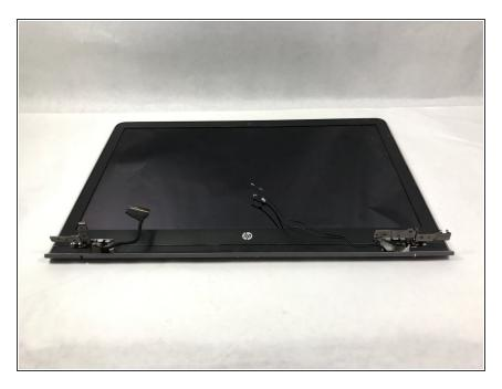
Once these steps are completed, you may lift the display assembly free from the rest of the device.
