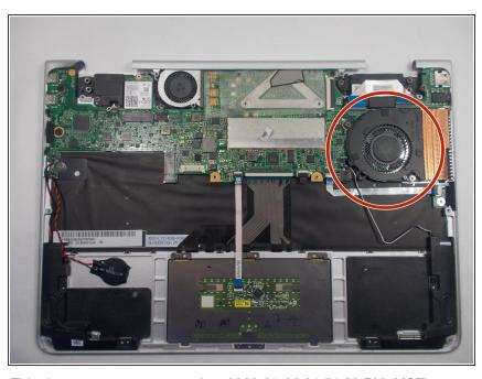
Locate the Cooling Fan in the device.
