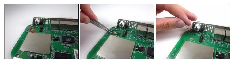
• Use <u>tweezers</u> to gently pull the metal bracket that connects the antenna to the motherboard.
