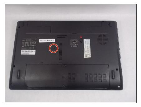
Remove the M2.5x8 screw using a Phillips #0 screwdriver.
