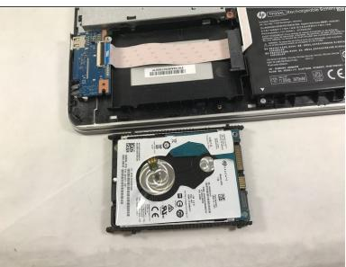
Carefully remove the connector ribbon cable from the elevated end of the hard drive, then remove
