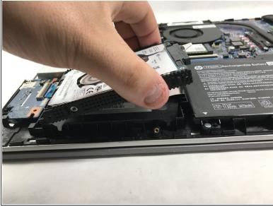
Using a spudger or the opening tool, lift the end closest to the battery until you can hold the hard drive with your hands.
