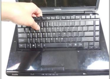
• Starting at the top, gently raise the keyboard enough to remove it from the socket.
