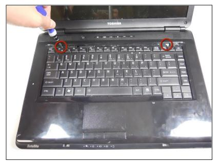
Remove the two 4.8 mm screws from underneath the plastic cover piece using a Phillips #00 screwdriver.
