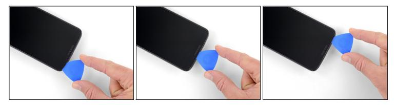
• Slice through the glue under the lower bezel.
