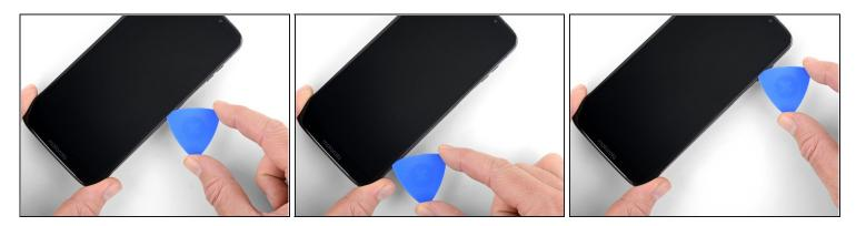
Slide the tool all along the right edge of the phone to slice through the adhesive securing the display.
