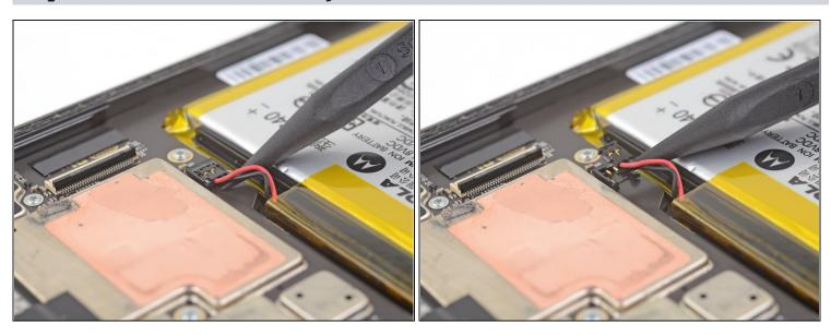
• Use the point of a spudger to pry the battery connector straight up and disconnect it.
