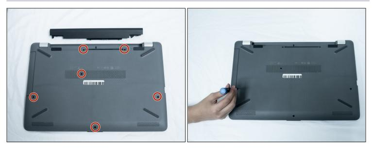
• Use a Phillips #0 screwdriver to remove the six 10.5 mm screws visible on the bottom of the laptop.
