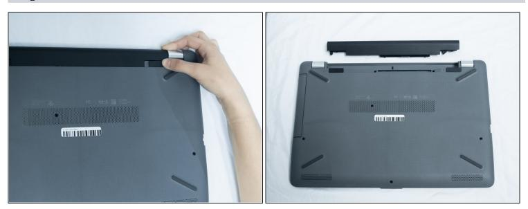
• Slide the Battery release slider towards the battery while pulling the battery out.
