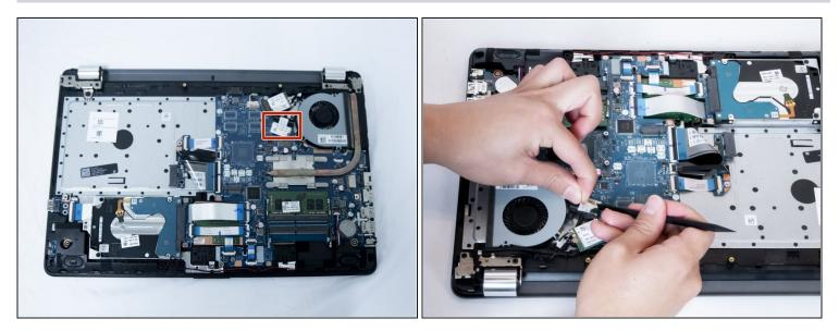
• Carefully unplug the LCD connector using a plastic spudger.
