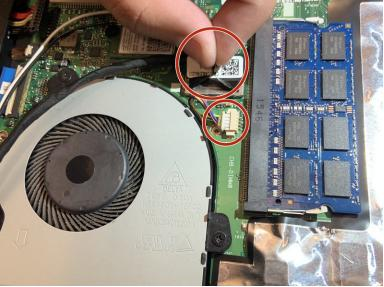
Disconnect the two cables connecting the fan to the motherboard.
