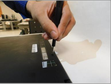
• Remove the ten circled screws along the perimeter of the laptop with a Phillips #0 screwdriver.
