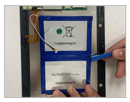
Once you remove the battery, simply replace the battery with a new one.
