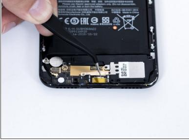
Remove the two 3.8mm Phillips #0 screws holding down the lower metal bracket.
