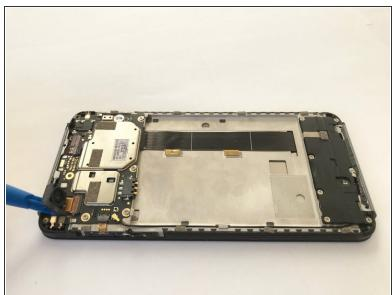
Use the plastic opening tool to lift the camera out.
