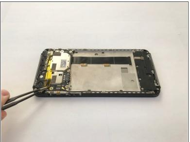
Remove the yellow plastic tape using a pair of tweezers.
