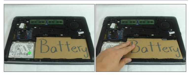
• Gently lift up on the battery (represented by this cardboard cutout) until it disconnects. Once the battery is disconnected lift away from laptop.
