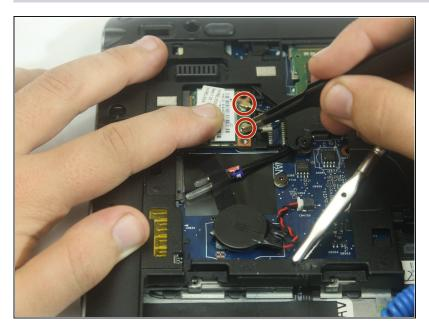
• Using precision tweezers grab the coaxial cable leads and disconnect them using steady gentle force.
