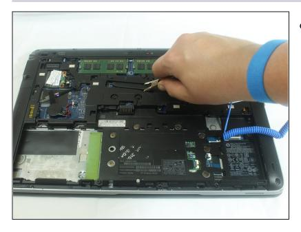
Attach the <u>anti-static wrist</u> <u>strap</u> to any metal piece on the computer to prevent electrical damage.
