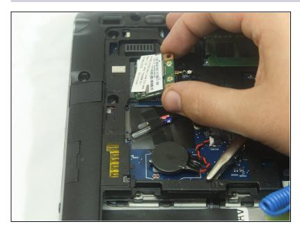
• Using the Phillips #0, remove the 1.5 mm screw holding the wifi card in place. Once the screws are removed, gently lift the card away from laptop.
