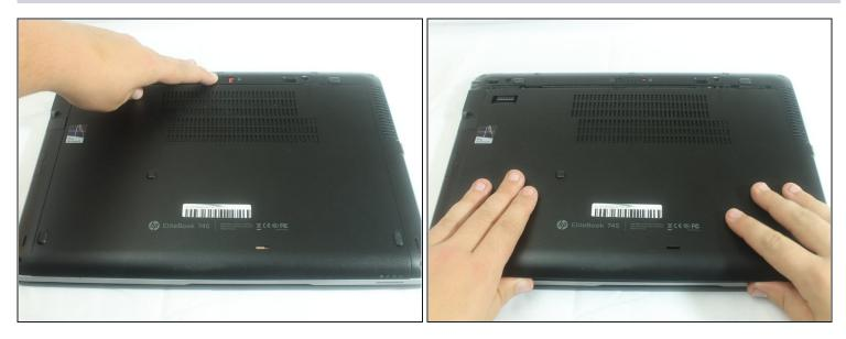
• Remove the cover by sliding the lock to the left. You will hear a click once the cover has been unlocked. Gently push down on the cover and slide it towards you to remove it.
