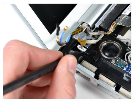
Disconnect the inverter cable from the left I/O board by placing a spudger beneath the cable and lifting up.
