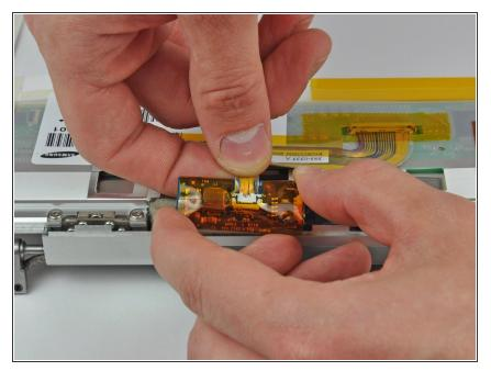
• Disconnect the backlight cable by pulling its connector away from the socket on the LED driver board.
