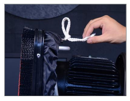
• Untie and loosen the drawstring securing the dust skirt.
