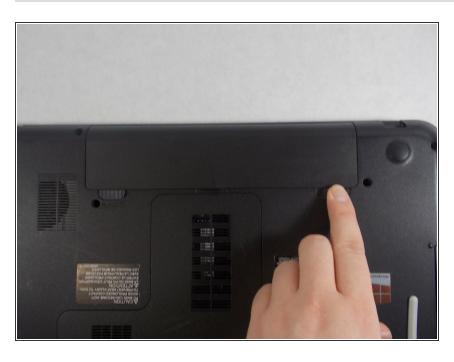
Move the right notch to the unlock position by sliding it to the right.
