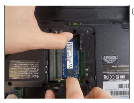
Line up the new stick of RAM with the gold contacts facing the slot and evenly push the new stick into the same slot which you removed the old stick.
