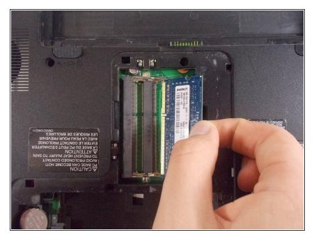
Carefully hold the edges of the RAM and remove the stick.
