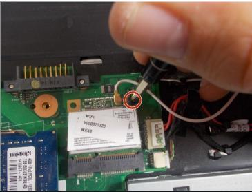
• Remove the single screw securing the Wi-Fi card using a Phillips #0 screwdriver.
