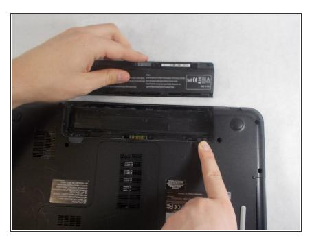
Hold the left notch in an unlocked position with one hand and use the other hand to slide the battery out.
