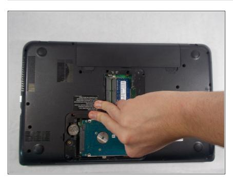
Grasp the side of the hard drive opposite the circular battery, and carefully pull out the drive by moving it away from the circular battery.
