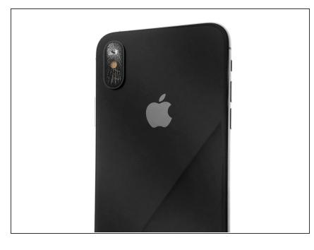
• To begin with, it will be necessary to remove the pieces of glass from the old broken camera lens.
