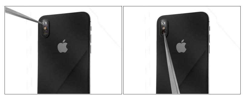
Once the glass shards from the camera lens are removed, thoroughly clean the camera bezel (the raised metal part around the camera).
