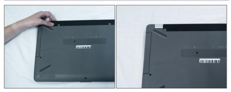
• Slide the Battery lock slider to the right until you see the "Unlocked" lock symbol.
