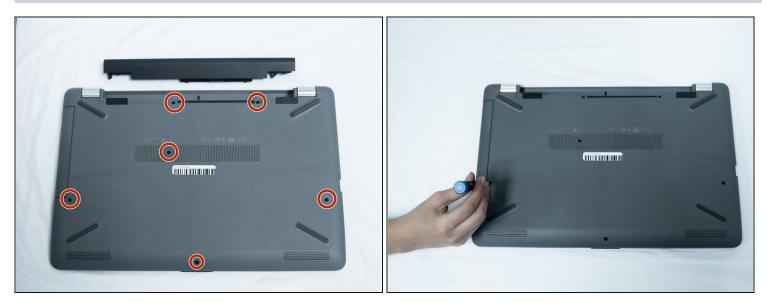
• Use a Phillips #1 screwdriver to remove the six 10.5 mm screws visible on the bottom of the laptop.
