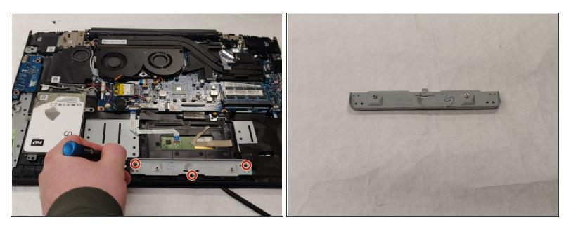
• Using the Phillips #0 screwdriver, remove the metal reinforcement by removing the three screws.
