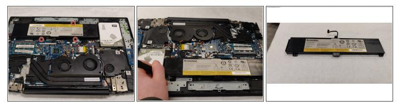
• Using the Phillips #0 screwdriver, remove the three screws holding down the battery.
