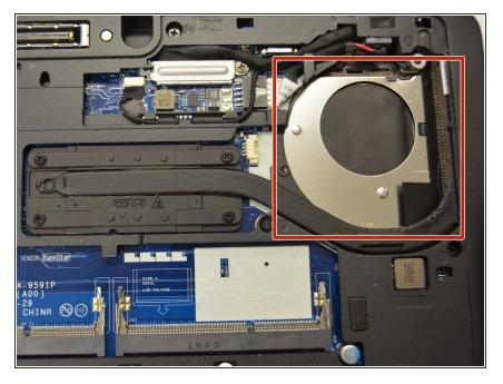
Remove the fan from the device.
