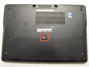
Slide the latch and remove the battery.
