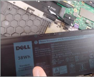
• Pull the plastic tab on the battery cable to disconnect the cable from the battery.
