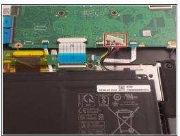
Remove the ribbon cable by pulling the plastic connector that is connected to the motherboard out.
