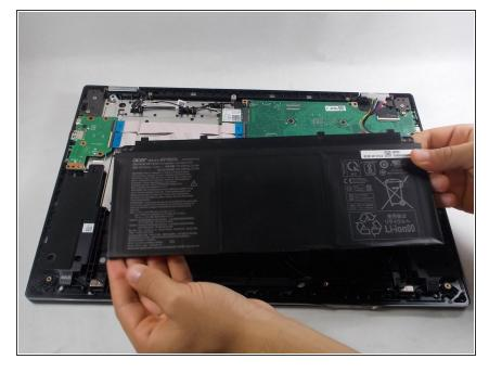
Remove the battery from the laptop by hand.
