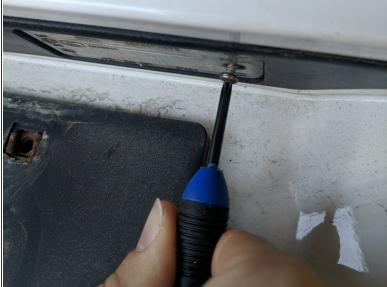
Using a small screwdriver, loosen and remove the screw that is holding the license plate light in place with a Phillips #1 screwdriver.
