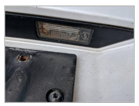
Open the hatchback and hold it in place so that you can easily reach the lights that illuminate the license plate. You may need to have another person hold the hatchback steady for you.
