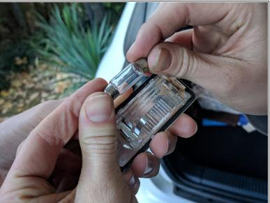
Use one hand to hold the light steady. Place the thumb and the index finger of the other hand on the metal ends of the light. Gently pull the light away from the metal frame.
