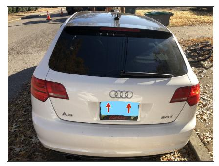
i The red arrows point to the relative location of the license plate lights (under overhang of hatch door where license plate is).
