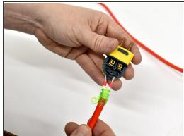
Loosen the screw terminals to remove both cable ends. They are not polarity specific (side does not matter). The screws just need loosened, not removed.
