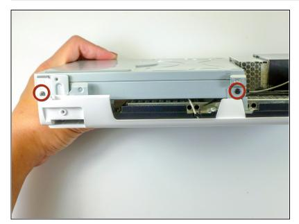
On each side of the DVD drive, remove the two 4.6mm Phillips #0 mounting screws.
