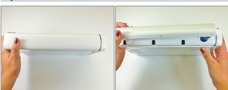
• On the side opposite of the exhaust vents, slide the cover faceplate towards the back of the console and pull upwards to release it.
