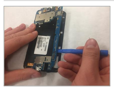
Place the plastic opening tool between the blue motherboard and black plate and pry until the motherboard pops off.
