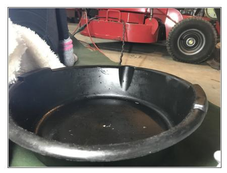
Place a drain pan underneath the fuel filter to collect any excess fuel that leaks from the fuel filter and lines during disassembly.
