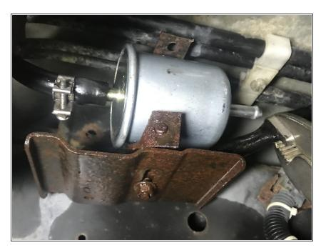
Put the fuel filter back in the clamp.
