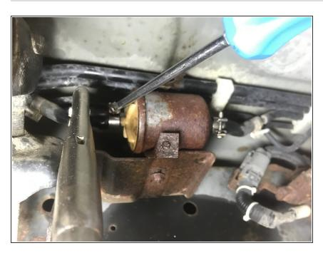
Using a Phillips 3 screwdriver, loosen the screws on the hose clamps located on both sides of the fuel filter.
