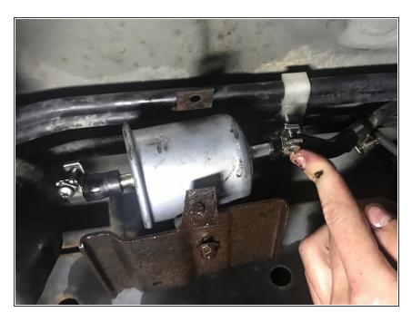
Slide the hose clamps back on the fuel filter fittings over the fuel lines on both sides of the fuel filters.
