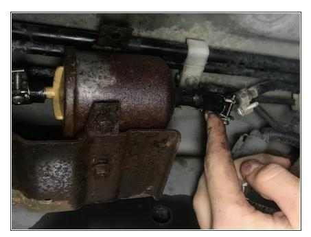
Slide the fuel line clamps off both sides of the fuel filter fittings.
