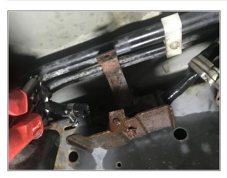
Remove the old fuel filter from the clamp in which it should slide out since it is already loose.
