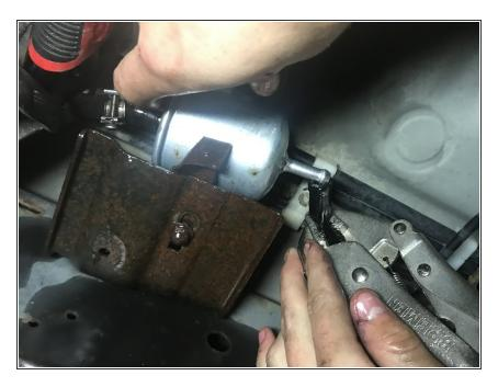
Place the other fuel line on the fuel filter fitting.
