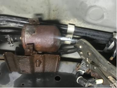
Using a flat head screw driver, work loose the fuel line if it has been on the fitting for many years.
