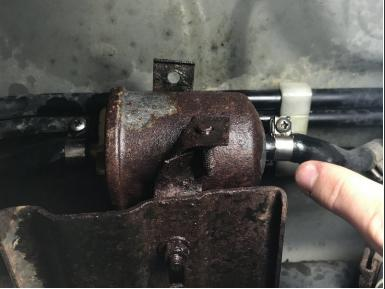
• Locate the fuel filter under the passenger side of the cabin, mounted on the inside frame rail.
