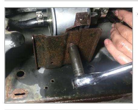
Using the 10 mm socket wrench, tighten the clamp that holds the fuel filter into place.
