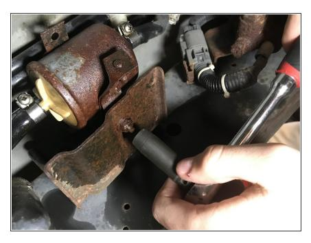
Using the 10 mm socket wrench, loosen the bolt on the clamp that holds the fuel filter in place.
