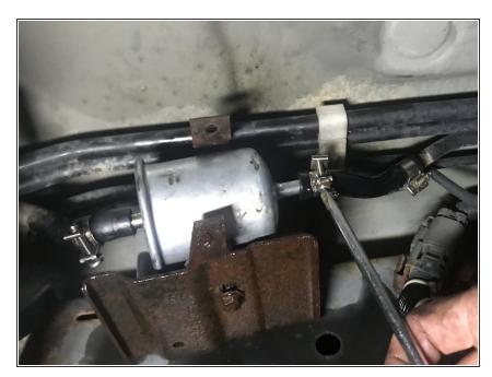
Using the Phillips 3 screwdriver, tighten the hose clamps on the fuel line until it is tight without over tightening cutting the fuel line.
