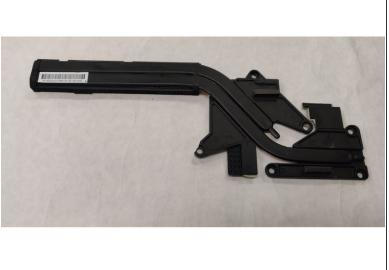
Using the Phillips #0 screwdriver, remove the six screws holding down the cooling unit.
