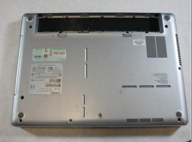
Pull the battery out by lifting the battery cover away from the laptop.
