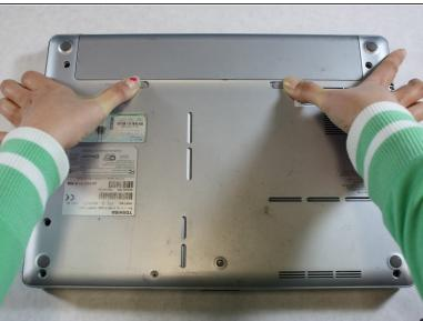
Slide both of the latches to the outside to release the battery.
