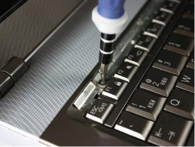
Using your Phillips #00, unscrew the two 4.80mm screws at the top of the keyboard.
