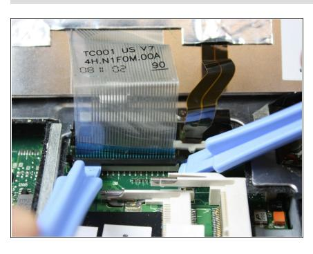
Using the plastic opening tools, pop out the ribbon cable from the rest of the computer.
