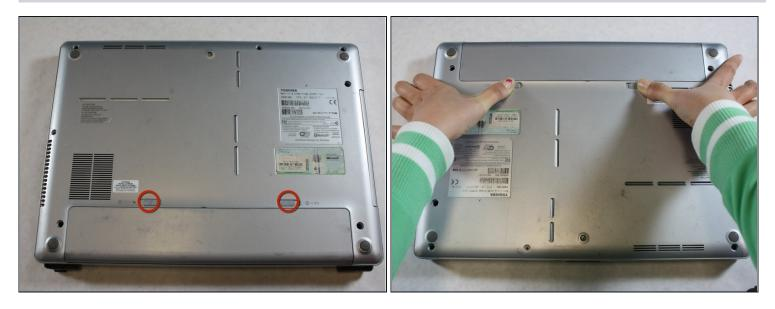
Slide both of the latches to the outside to release the battery.
