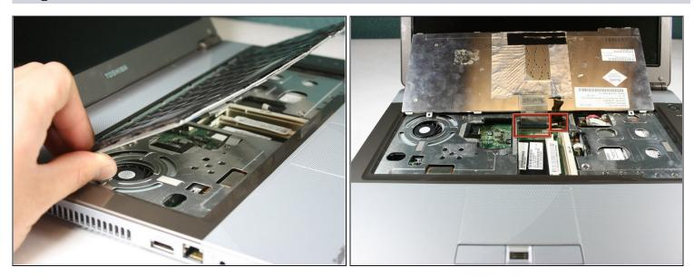
⚠ When removing the keyboard, be careful not to rip the ribbon cable connecting the keyboard to the computer, to avoid damaging it.
