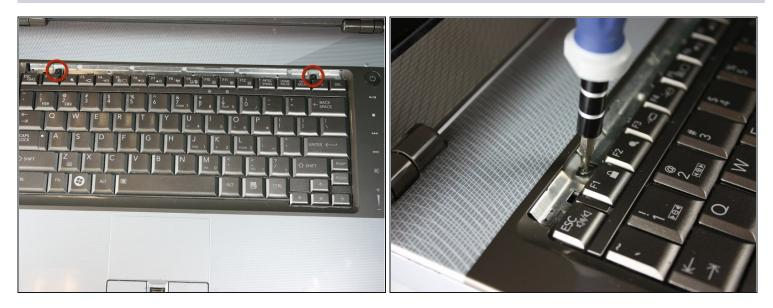
• Using your Phillips #00, unscrew the two 4.80mm screws at the top of the keyboard.
