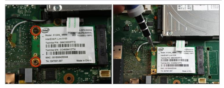
• Locate and remove the two Philips #00 4.85 mm screws on the left of the WiFi card.
