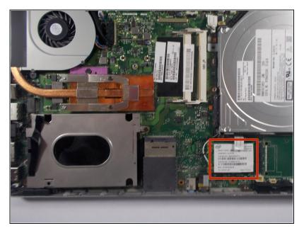
Locate the WiFi card, which is directly beneath the disc drive.
