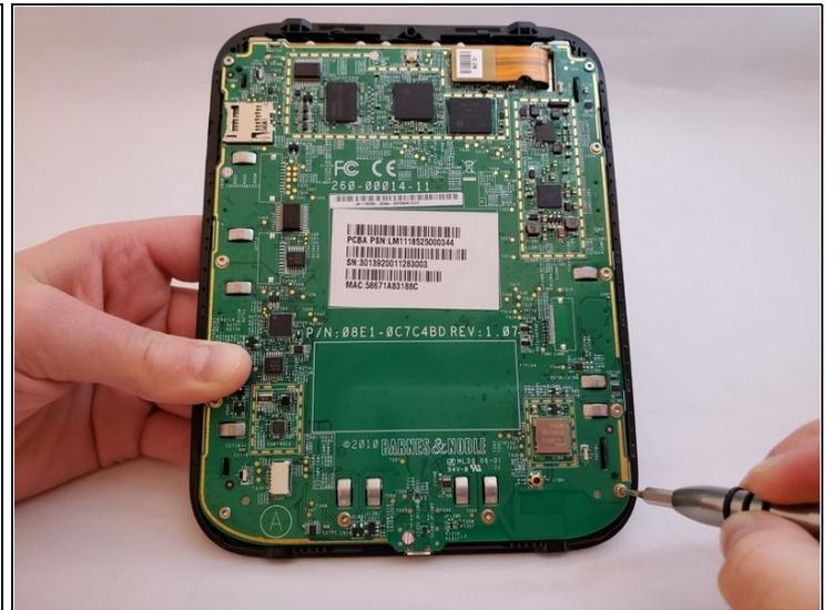
⚠ Use an anti-static mat to prevent electric shock from damaging the motherboard and its components. Be careful when using metal tools on your device.
