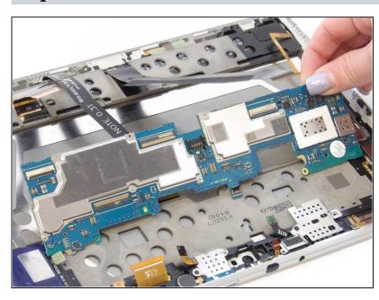
Remove the motherboard by gently sliding it out of its casing.
