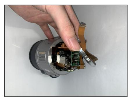
The outer casing of the lens consists of two outer casings that are secured by an end cap that connects them. In this part we take this end cap
