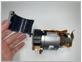
Place the lens section horizontally on the workbench and pry open the top cover of the lens with some effort
