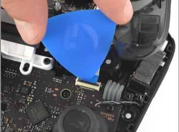
• Use the tip of an opening pick to open the black flap of the ZIF connector by pushing it upwards.
