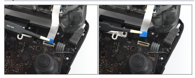
• Use your fingers or a pair of blunt nose <u>tweezers</u> to disconnect the interconnect cable from its connector.
