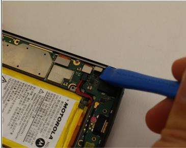
Using the iFixit opening tool, pop up the three press-fit connectors in the bottom right corner of the motherboard.
