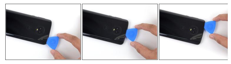
Slide the pick all along the top edge of the phone to slice through the adhesive securing the rear glass.
