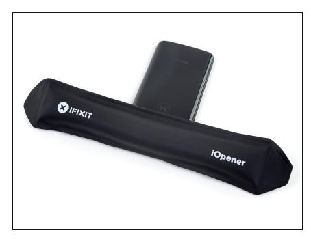
Heat the top edge of the back of the phone to soften the rear glass adhesive.
