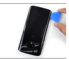
Slide a pick along the left edge of the phone to slice through the rear glass adhesive.
