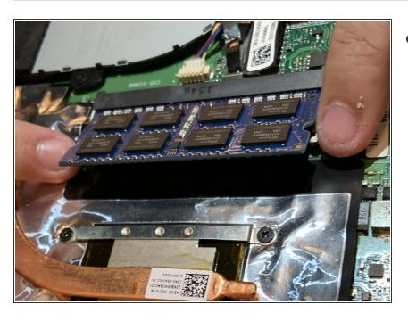
Upon unlocking the mechanism, you should find that the component now pops up at an almost 45-degree angle. Lift it up gently and carefully.
