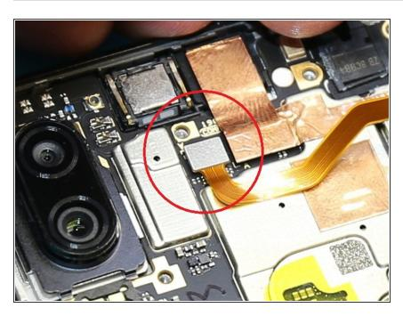
Pry up on the connector and remove the fingerprint sensor cable.
