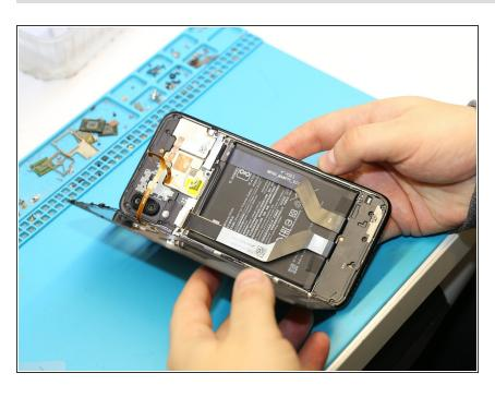
Lift the cover open like a book, but be careful to make sure you do not damage the flex cable while it's still connected.
