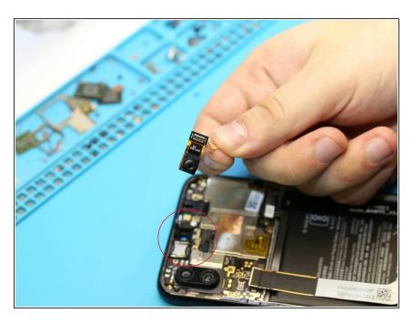
Disconnect the connector on PCB, and remove the front facing (selfie) camera.
