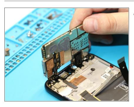
Pull off and remove the PCB.
