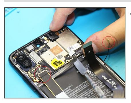
Disconnect the connectors on the PCB.
