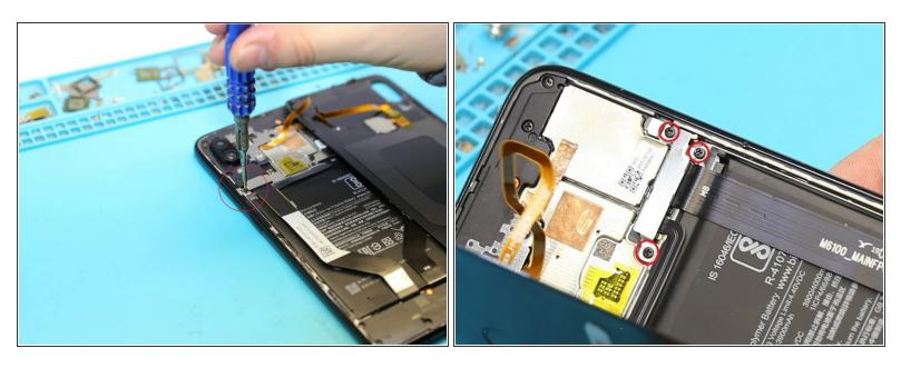
• Using a screwdriver (1.5 mm), unscrew 4 screw and remove the bracket holding the connector.
