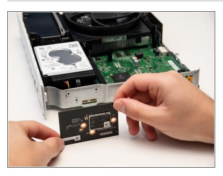
Carefully remove the WiFi Card from the metal chassis.
