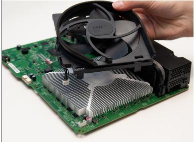
Lift the fan away to fully remove it.
