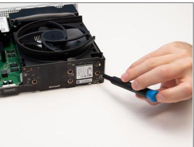
Remove the four 15mm screws attaching the IR Blaster to the metal chassis with the Torx T8 Security screwdriver.
