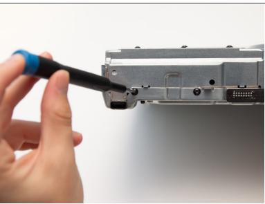
Remove the two 15mm screws from the front panel using the Torx T8 screwdriver.
