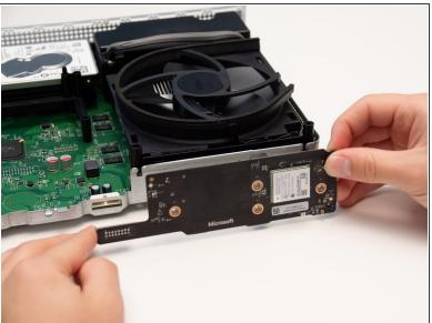
Carefully remove the IR Blaster from the metal chassis.
